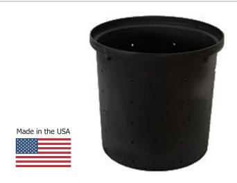
The SF15-DR is the perfect basin for crawlspaces or where space is limited. It incorporates our heavy duty, non-corrosive nylon encapsulated inserts. This basin has a total capacity of 15 gallons. Constructed from ultra strong, heavy duty structural foam, it will provide decades of reliable service. It is factory perforated with 40, 5/16" holes that allow for a quick reduction of standing water in crawl space areas, yards patios and driveways.
